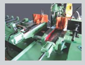
Nesting Fixture is provided for cutting small size bars by stacking/bundling with an additional top clamping.
