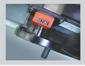
The hydraulically operated rear vice mounted on a slide, moves bar stock forward as per the preset length.
