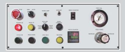
The Bandsaw has a Centralized Control Panel, conveniently positioned on right side of operator.
