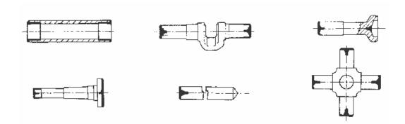
CNC Centering & Plunge Facing machine are suitable for centering and plunge facing at both ends, simultaneously of the bar stock. The combined centering and facing operation saves machining time, handling time & floor space.
